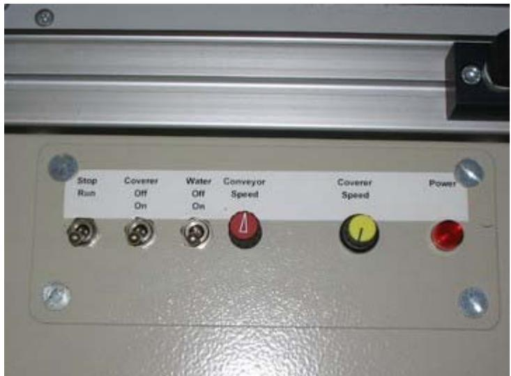
Switch on the water bar, and run another test tray through. Adjust the volume of water using the regulator. Turning counter-clockwise increases water flow.
