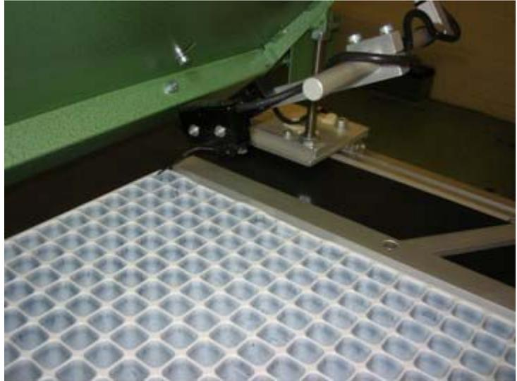
Adjust the height of the water bar so that the tips of the nozzles are around 12mm from the top of the tray.
