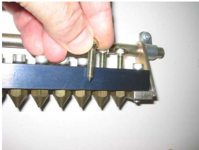
The seed discharge tubes have both ends machined inside to a taper, to help prevent seed hang-up. If the tubes have to be shortened, ensure the tapered end is fitted into the profile bar.
